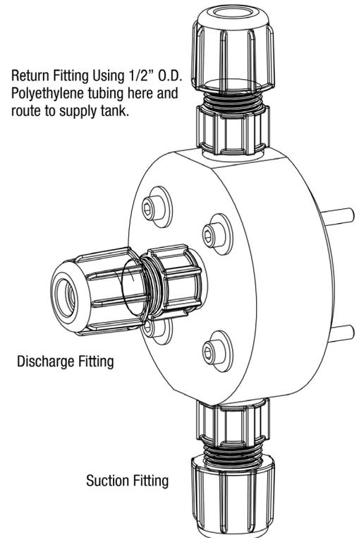
The AUTOPRIME™ valve allows the pump to prime during pump start-up, when gas or air binding is a greater risk. It also continuously vents gas that may form during normal pump operation.
